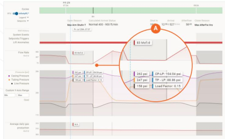
**A** A flow reading (83mcf/d) in the offtime indicating a flow meter error.
