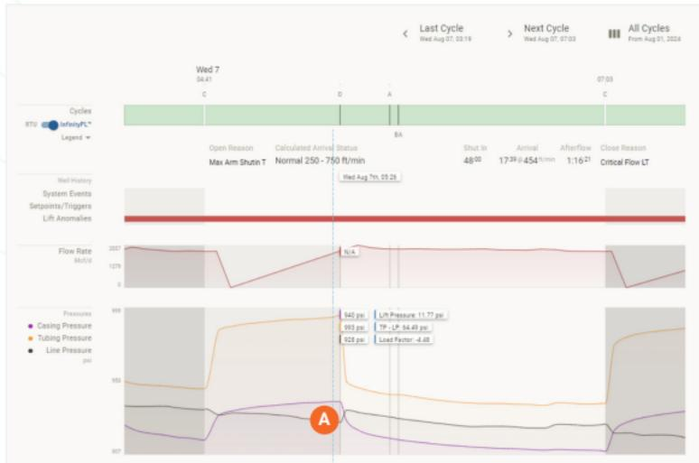
**A** Casing reads lower than tubing or line, even though the trend through the cycle looks normal.
